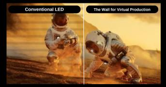
By supporting an industry top level 12,288 Hz refresh rate, The Wall for Virtual Production minimizes flicker lines and artefacts when shooting the image on display through a camera.
