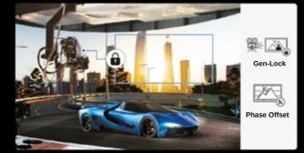
The Wall for Virtual Production allows to genlock all the signals of the entire system, ensuring a perfect synchronization. It also offers a phase offset function for further frame corrections.
